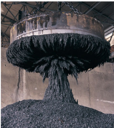
Figure 28-1 Using an electromagnet to collect and transport scrap metal at a steel mill.
